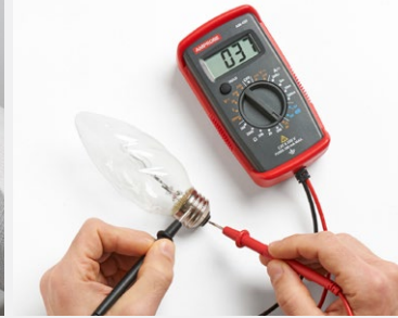
Troubleshoot light bulbs and fuses with the continuity function
